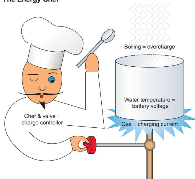
A PWM controller holds the voltage more constant. If it has two-stage regulation, it will first hold the voltage to a safe maximum for the battery to reach full charge. Then it will drop the voltage lower to sustain a “finish” or “trickle” charge. Two-stage regulating is important for a system that may experience many days or weeks of excess energy (or little use of energy). It maintains a full charge but minimizes water loss and stress.
