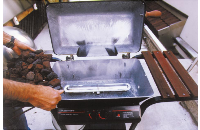
Above: By removing the cooking grill and lava rock support, you can see the stainless steel propane burner.
