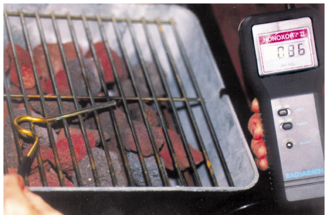
Above: Test setup showing barbecue, NOx meter at 50% hydrogen flow (86 ppm)
