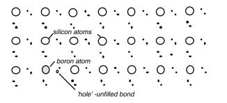
Figure 3 p type (boron) doped silicon
